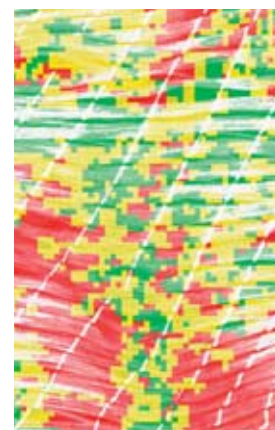
Automated testing of angularities on multi-axial layings with digital image analysis
