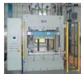
Deformation pressing for processing fiber-reinforced thermoplastics
