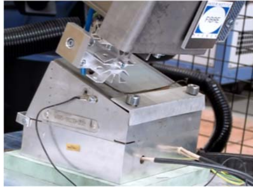
Figure 2: Prototype of printing-head while printing 3D-structures
