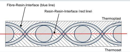
Main principle of the hybrid matrices with woven interlayer
