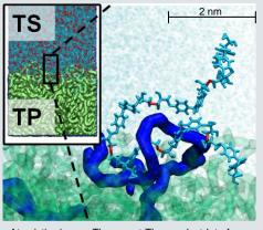
Atomistic view on Thermoset-Thermoplast-Interface (TS/TP) based on Molecular Dynamics Simulations
