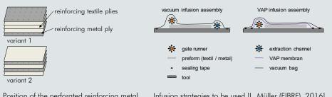
Position of the perforated reinforcing metal ply in the laminate
