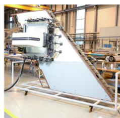
Figure 2: Milling robot on the vertical fin
