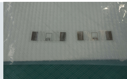
Left: Examples for different sensor geometries Right: Sensors on woven fibres
