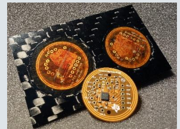
Electronics of actuator. Embedded antenna with PWAS and battery-less NFC/RFID Temperature Sensing Evaluation.
