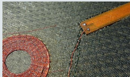
Electronics of actuator. Embedded antenna with PWAS and battery-less NFC/RFID Temperature Sensing Evaluation.
